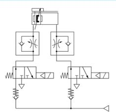
This control circuit improves the positioning accuracy. The use of check valves reduces the stopping distance and also increases the load stiffness.
