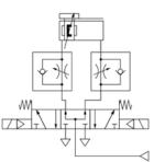
System to stop the cylinder on intermediate position with higher tolerances.
