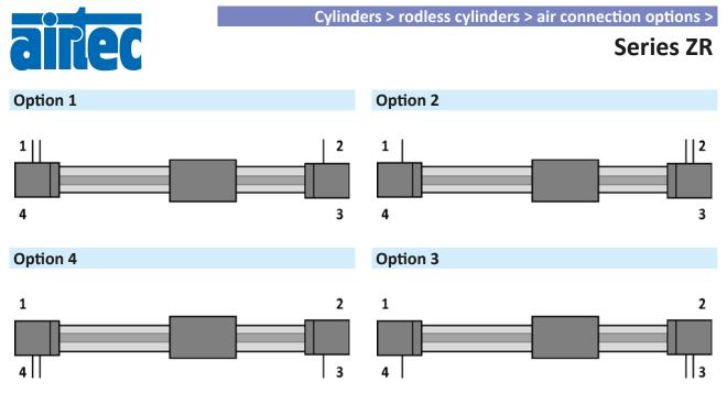
The cylinder is supplied with three air connections. Two connections are necessary for operation, while the third is closed by a plug (included in the scope of delivery). The desired position of the double connection has to be specified in the order code after the stroke length by choosing the adequate number.
