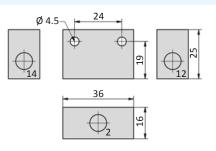
12, 14 = signal input 2 = signal output
